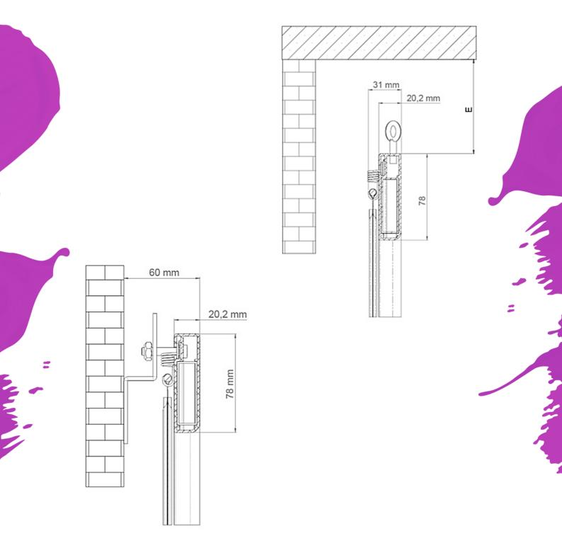
Screen section and dimensions with optional bracket for wall mounting
